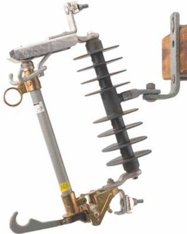
A sharp downward pull on the lever with a hookstick breaks the fuselink. (15/27 kV product shown here)
