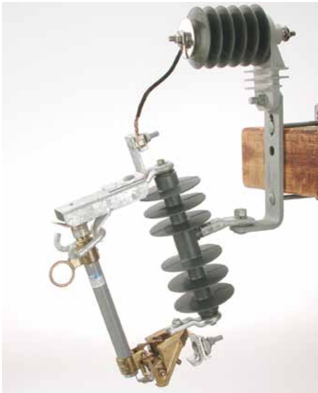
15 kV cutout with direct-connected Ohio Brass MOV, polymer 9 kV lightning arrester
