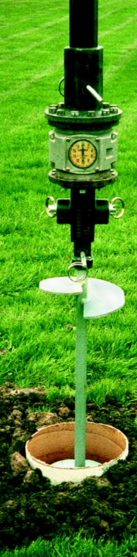
Displacement plates form grout column to design depth
