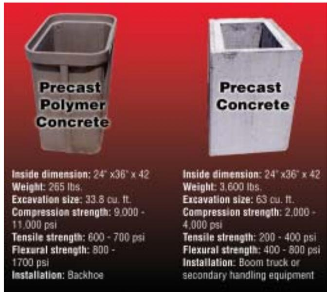
Compared to precast Portland cement concrete, precast polymer concrete is lighter in weight, stronger and more cost effective to install because the equipment used to dig the hole can be used to set the enclosure..
