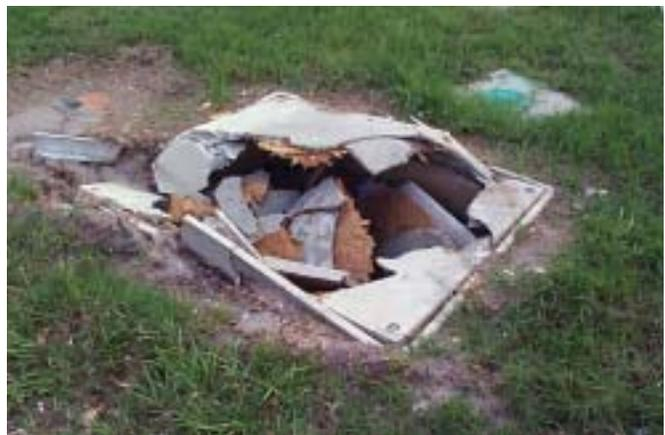
Sprayed-up fiberglass and wood make up this failed dissimilar materials enclosure. Lack of strength was an obvious issue in this application.
