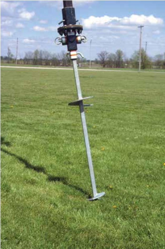
However, it is easy to observe, even without gauges, when one specimen strikes an obstruction and another does not. Specimens should be installed under conditions as nearly identical as is possible. Obviously dissimilarities in the test media exert different mechanical stresses on the anchors which will be reflected in tension or compressive loading capabilities.
