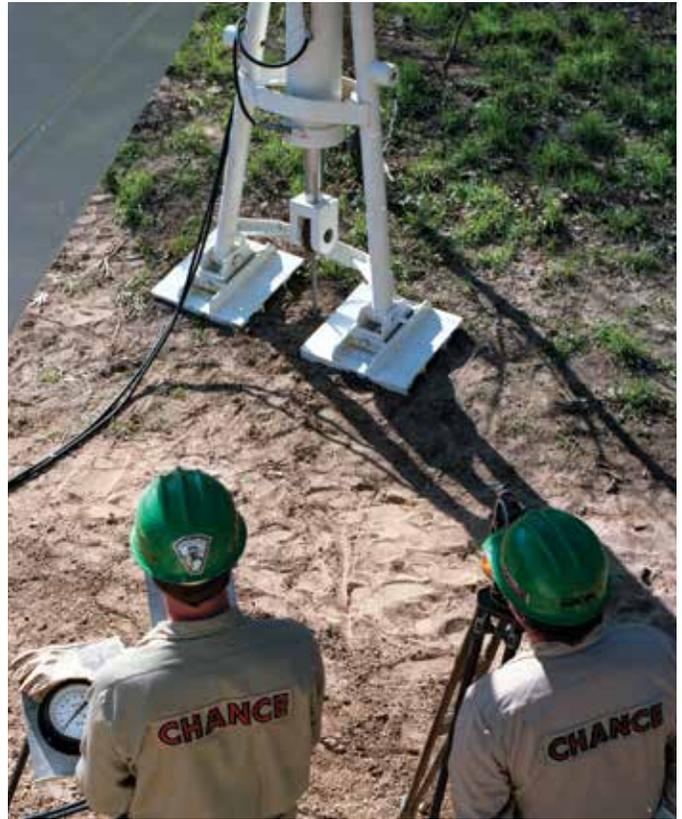
Typical anchor test set up.
