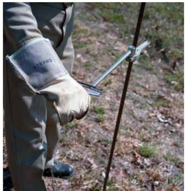
The Chance Soil Test Probe enables quick identification of the sub-soil to properly mate anchor and holding requirements.
