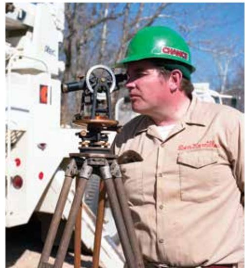
Transit is used to measure anchor creep.
