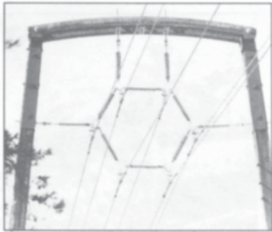
6-phase Ohio Brass Hi*Lite insulators on test line
