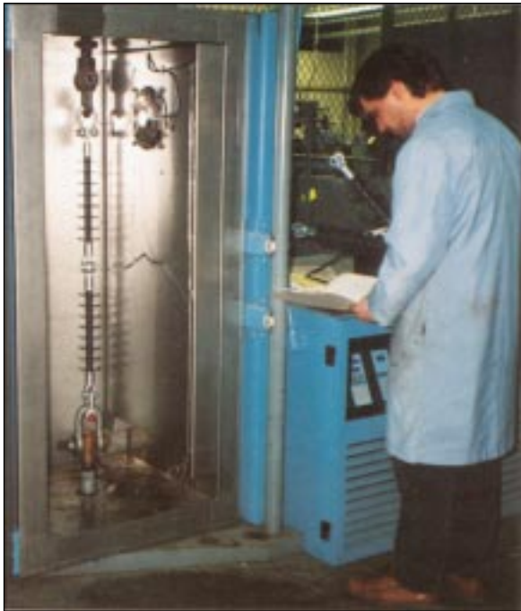
The temperature-pull tests verify the crimp strength is not affected by temperature.
