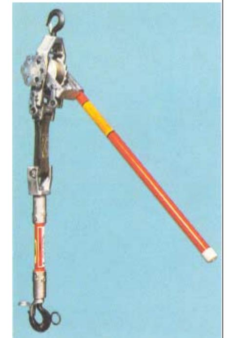
**"... one of the handiest tools a lineman can use. With a small investment in an insulated link stick, the hoist makes an even more valuable tool for rubber glove work."**
