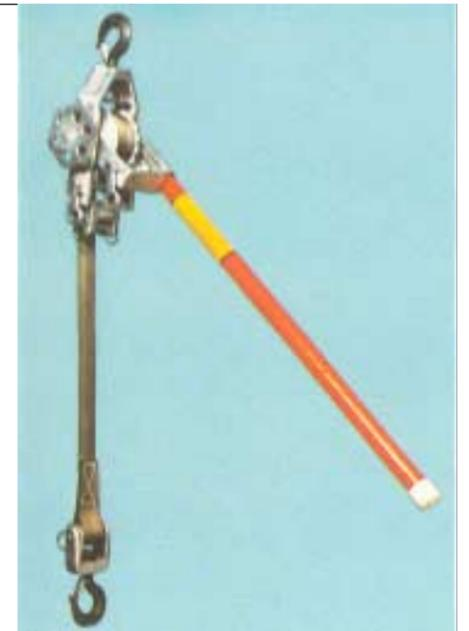
**Convertible hoist simply rigs to 3/4-ton rating by pulling sheave pin to remove hook from strap becket. This gives the hoist a full 7-ft. reach, 3 ft. more than with it rigged for 1 1/2-ton capacity.**
