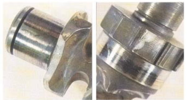
Shaft pocket damage.
