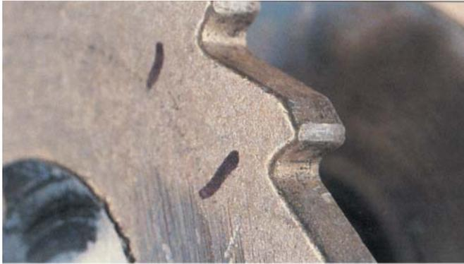
**Ratchet spool teeth — damaged from self ratcheting.**
