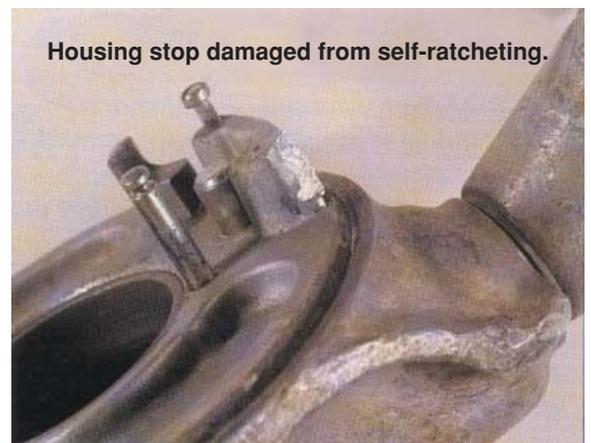
**Housing stop damaged from self-ratcheting.**
