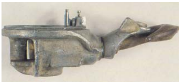
Housing with bent hook and stop damage.
