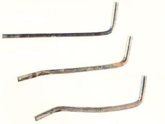
**Reversing rods — Top part is good. Bottom two parts bent.**
