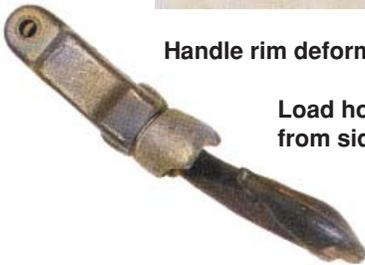
**Load hook assembly bent from side load.**
