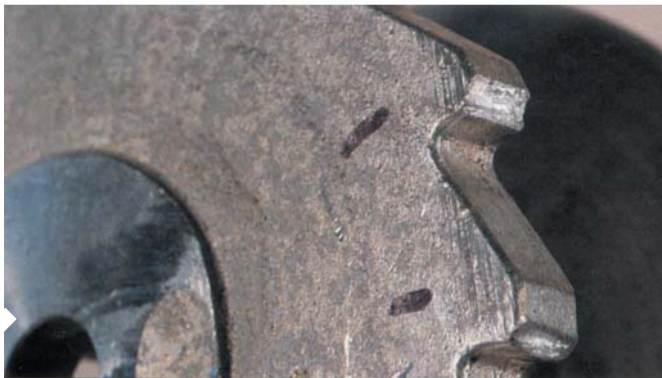
Ratchet spool teeth — sheared from overload or impact.
