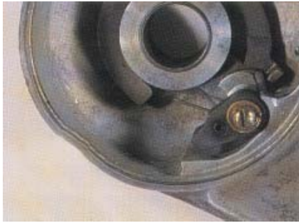
Handle rim deformed by dropping.
