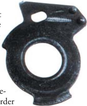
**Damaged unloader plate.**
