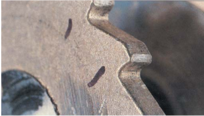
Ratchet spool teeth — damaged from self ratcheting.
