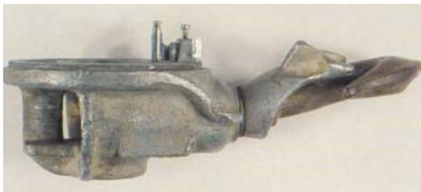
**Housing with bent hook and stop damage.**
