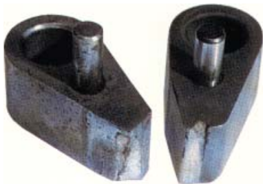
Dogs damaged by impact
