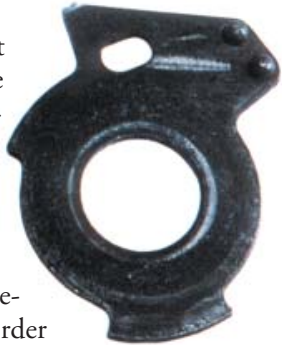
Damaged unloader plate.
