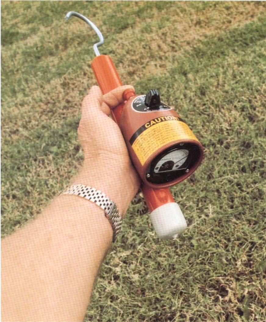
*Built-in pushbutton performs self-test. To make sure the MRVD and its 9-volt battery are working properly, OG&E makes this test before and after checking line voltage with the device.*
