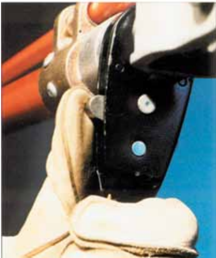
Selector switch on ratchet wrench is extra large for easy operation by hot-stick and rubber-glove methods.
