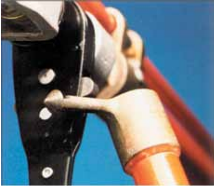
Selector switch on ratchet wrench is extra large for easy operation by hot-stick and rubber-glove methods.
