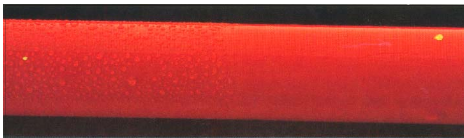
(Above) To pass the OSHA wet test, water must bead up rather than wet out the surface. Wax or silicone will enhance this property if the surface is in satisfactory condition.
