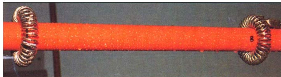
Close-up of the electrodes, below, and 1-foot test section. Note beading of water, indicating the stick surface is in good condition.
