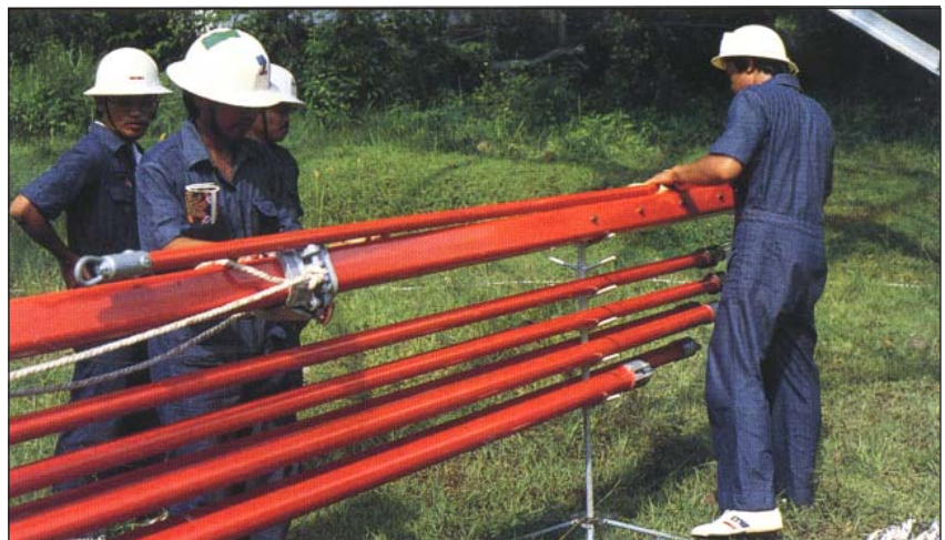
Used tool in basically good condition. With a wax or silicone wipe, this tool will pass the OSHA wet test and is satisfactory for service.
