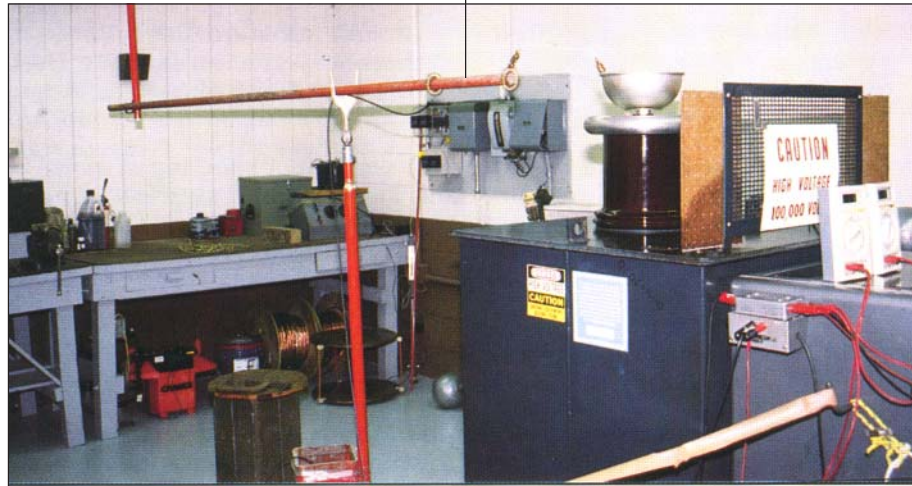
Typical laboratory set up for performance of the OSHA test. 75 kV is required for fiberglass tools: 50 kV is required for wood tools.
