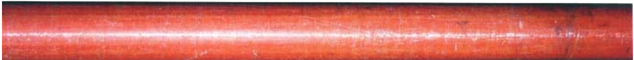
Typical used stick that will not pass the OSHA wet test even with a wax or silicone treatment. Complete refinishing is required to restore glossy surface and enable this tool to pass the OSHA wet test.
