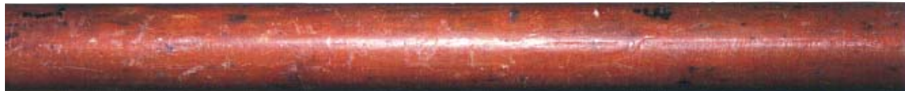
Tool as taken from utility service. This tool could not pass the OSHA wet test even after complete factory refinishing. Tools in this condition must be removed from service.
