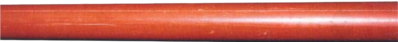
Used tool in basically good condition. With a wax or silicone wipe, this tool will pass the OSHA wet test and is satisfactory for service.
