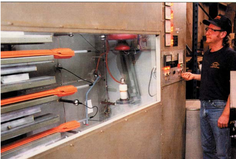
Electrically testing Chance cover-up prior to shipment.
