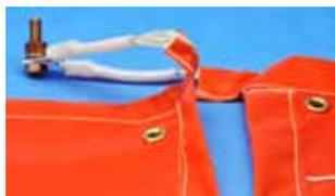
(At left) To join mats, the conductive grids simply connect at corner tabs with the bolt, washer and nut included with each mat. Tabs are fitted with shrink tube for stress relief. (Right) Ball stud can join mats and/or connect to grounding cable clamps.
