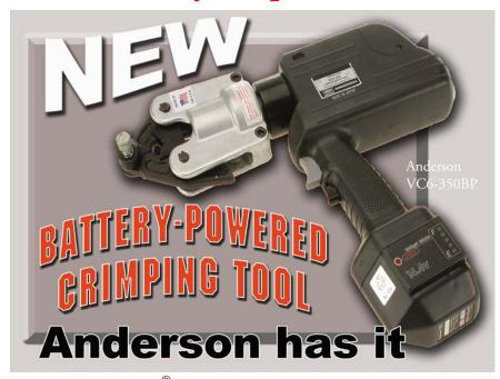
We've added further flexibility to our line of crimping tools with the VC6-350BP. It crimps lugs and splices to 350 MCM, and also includes a reversible "O" and "D" nib for H-tap connectors. Tool comes complete with impact resistant plastic case, battery charger, extra battery and three year warranty. Batteries charge in less than 25 minutes.
