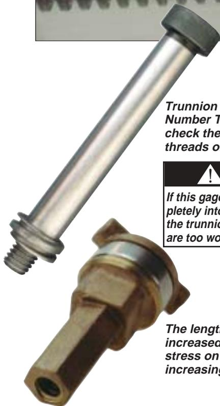
*Trunnion Gage, Catalog Number T401-2265, is used to check the wear of the internal threads of trunnions.*
