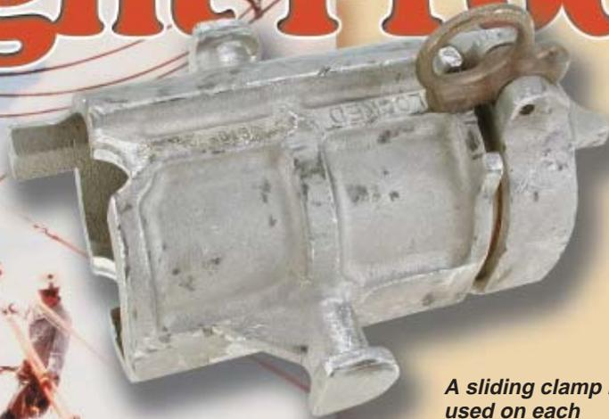
*A sliding clamp is used on each adjustable strain pole to place the bearing points at the proper spacing for the insulator string being worked. It slides on the pole and is positioned on the desired cross pin in the pole. The locking ring is then lifted and rotated to lock the collar against the adjacent cross pin.*
