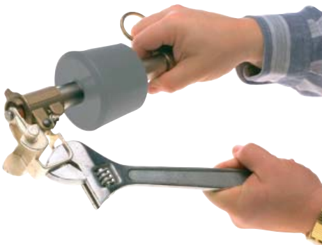
Figure 6 Resetting Chance Type CRS Sectionalizer
