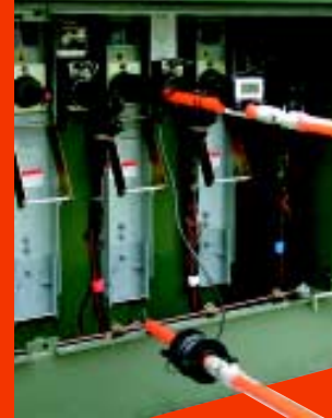
(Above left) Phase-phase voltage test, (above right) hi-pot test of cable with 16kV Kit's DC Hi-Pot Adapter between meter and bushing adapter (feed-thru device not included) and (at left) phase-to-ground test.
