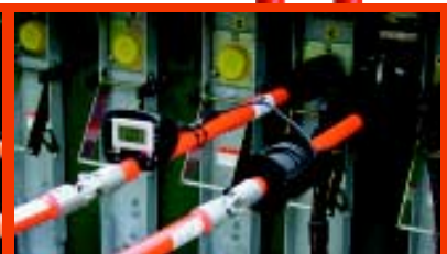
(Above left) Phase-phase voltage test, (above right) hi-pot test of cable with 16kV Kit's DC Hi-Pot Adapter between meter and bushing adapter (feed-thru device not included) and (at left) phase-to-ground test.
