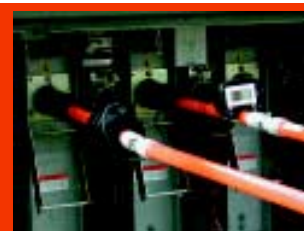
ARVI holds reading for voltage-indication tests on switch bushing (above) and cable (at right, using a feed-thru device).
