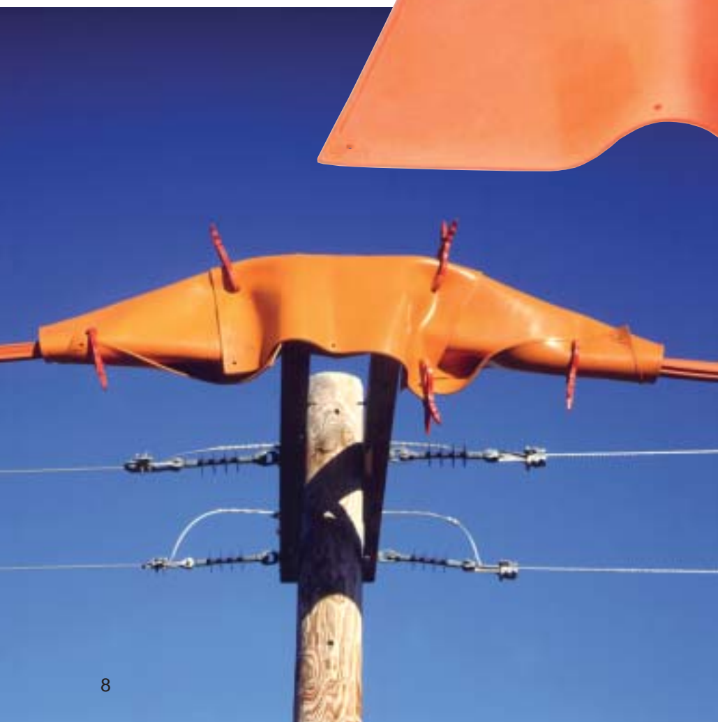
Chance solid and slotted blankets come in 36" x 36". Slotted blankets have a 1½"-diameter center hole to fit easily around common hardware.
