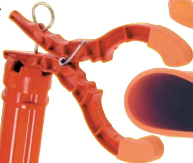
Chance clamp for Hotstick applications has rod loops for clampstick to capture and retract. Placement is easy and exact by either hot-line tool or rubber-glove method.
