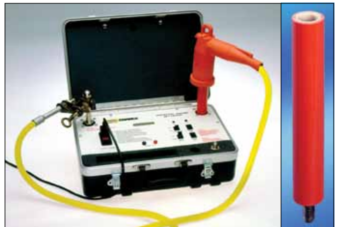
Optional Elbow Adapter C403-3449 for testing temporary grounding sets fitted with a grounding elbow.
