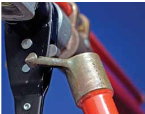
Selector switch on ratchet wrench is extra large for easy operation by hotstick and rubber-glove methods.
