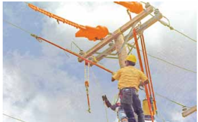
25kV Deadend Cover C406-0164 fits over a maximum of two 10"-diameter deadend insulators. Grip-All Adapter included allows placement with a clampstick or rubber gloves and sleeves when work practices permit.
