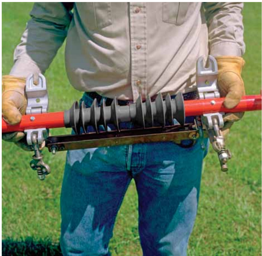
Locating pins in the Epoxiglas® pole ensure proper alignment of clamps for easy removal and replacement of switch hot parts.
