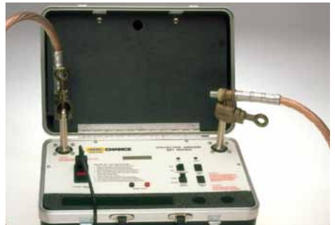
Ball-studs accept grounding sets with standard clamps (above) and Chance ball-socket clamps (below).
