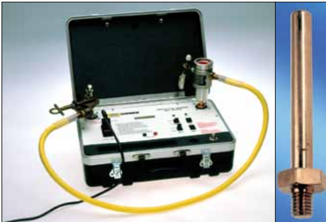
Optional Straight Stud Terminal T403-3159 for testing grounded-parking-stand temporary grounding sets.
