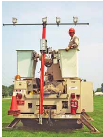
A scale on each side of monitor displays constant readout of load uplift for easy visibility from both buckets.
