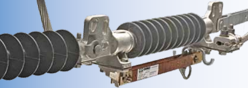
Catalog No. ALTD09200R 900A ALTD switch with side-mounted NEMA tin-plated copper terminal pads. The plated-aluminum end castings are for deadending only.
